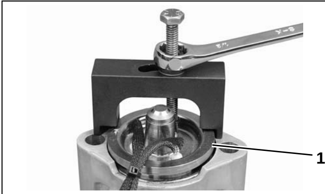
1. Fuel injector removed from fuel injector housing 008799
