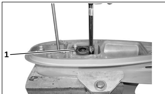
1. Driveshaft bearing housing
