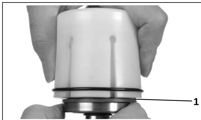
1. Seal installed in groove of piston
