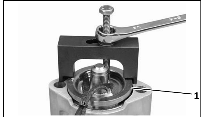
1. Fuel injector removed from fuel injector housing
