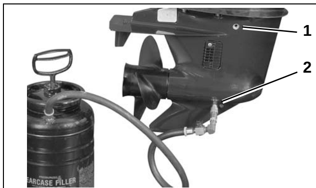
1. Lubricant level plug 2. Lubricant drain/fill plug
