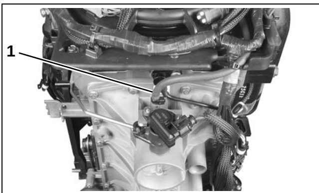
1. Vent hose connection to intake
