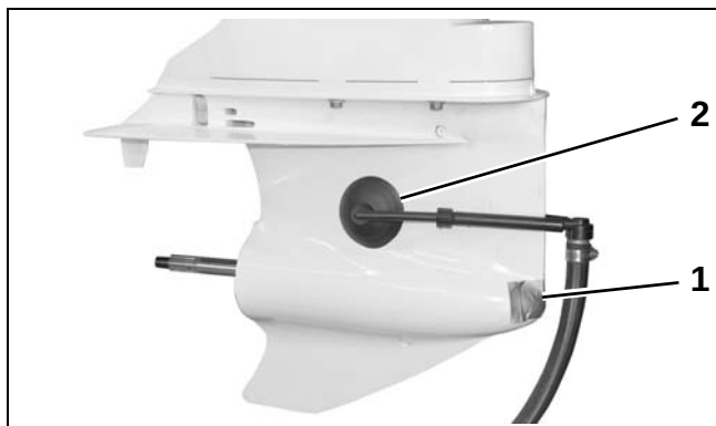
M2-Type Gearcase 1. Water-proof tape 2. Flushing adapter
