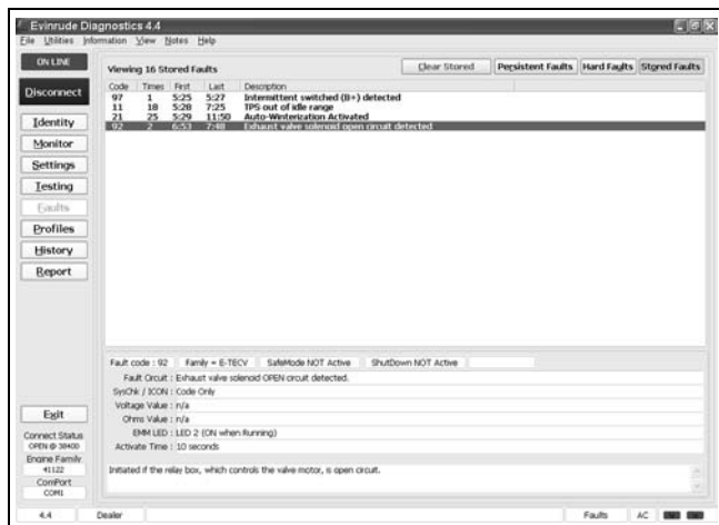
Stored Faults Review Screen
