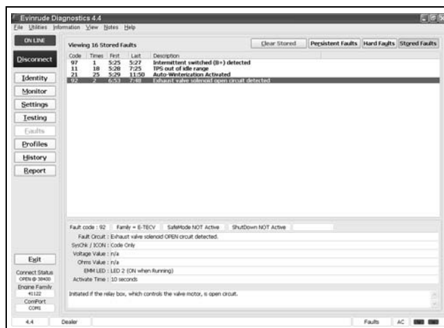
Stored Faults Review Screen
