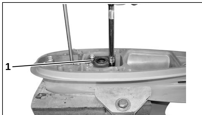
1. Driveshaft bearing housing
