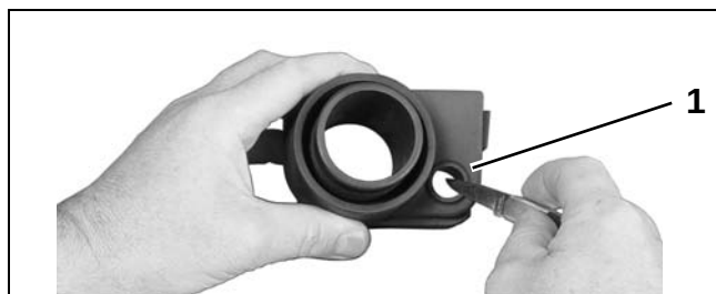
1. Alternate fuel hose location
