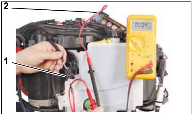
1. Oil injection pump connector pin A 2. EMM connector pin 2
