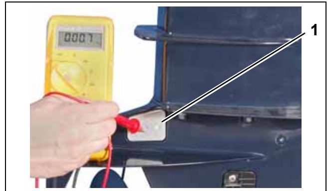
1. Meter lead to anode
