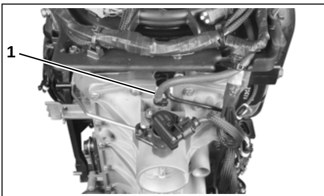
1. Vent hose connection to intake
