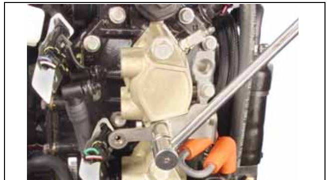
Tighten Screws in Stages
