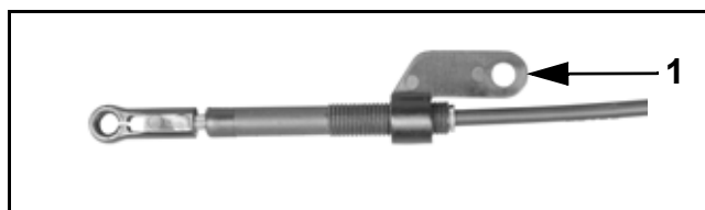
1. Turn anchor four turns toward cable end.
