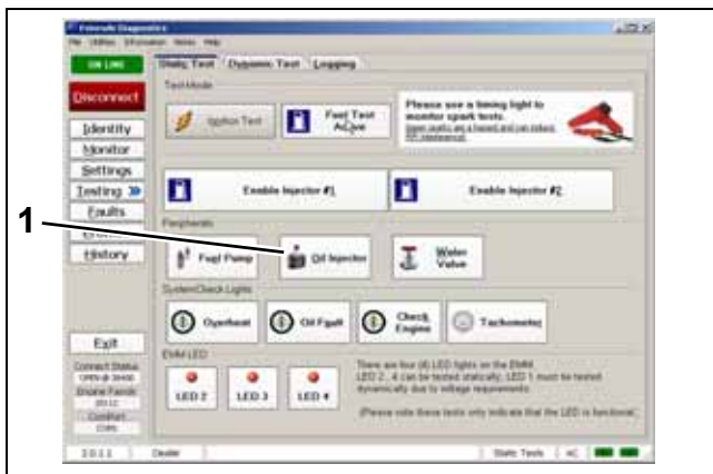
Static Tests Screen 1. Oil injector test button
