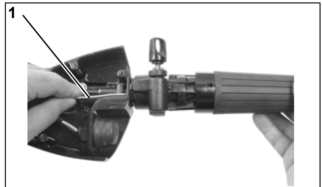
1. Trim switch wiring 006677
