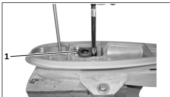
1. Driveshaft bearing housing
