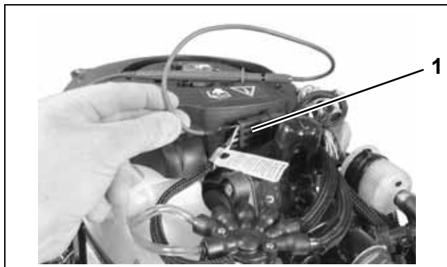
1. Oil injection pump connector (pin 1)
