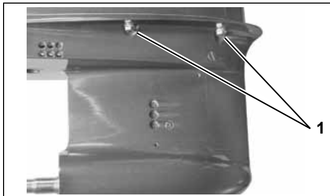
1. Gearcase retaining screws
