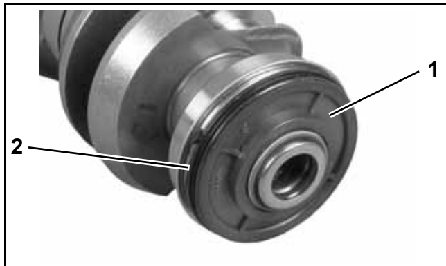
1. Lower seal housing 2. O-ring
