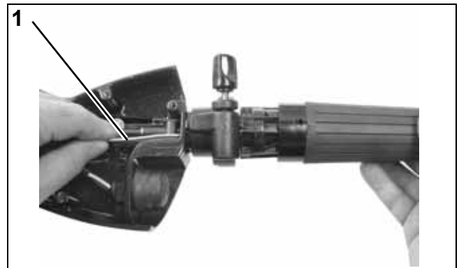
1. Trim switch wiring 006677
