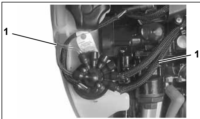
1. Oil distribution hoses
