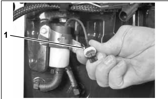
1. Water valve electrical connector
