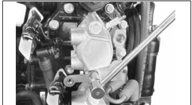
Tighten Screws in Stages
