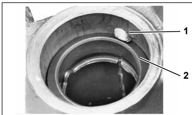
1. Steering friction pin 2. Steering friction thrust ring
