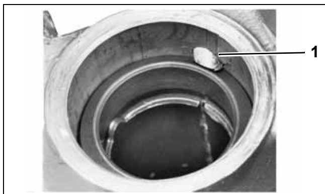
1. Steering friction pin
