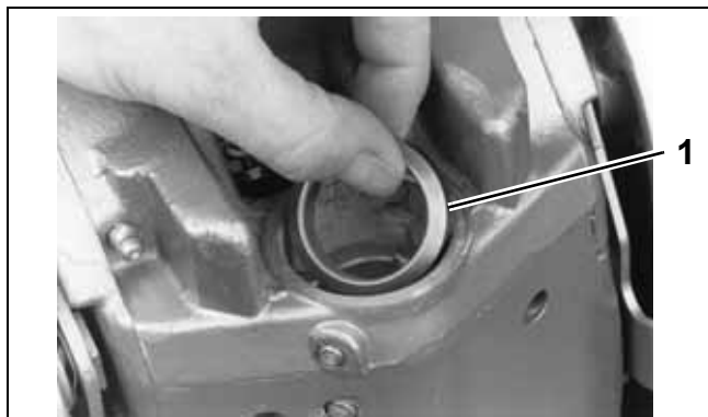
1. Steering friction thrust ring
