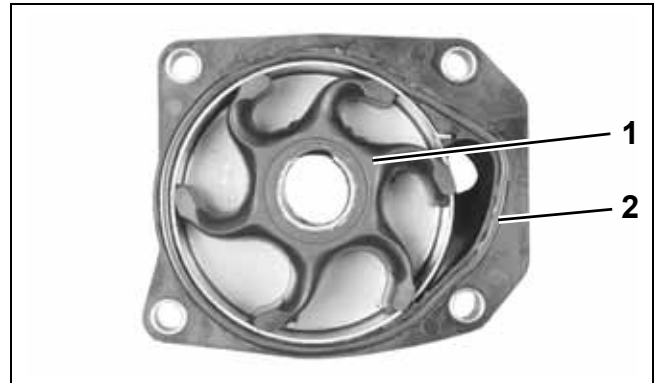
1. Impeller 2. O-ring seal
