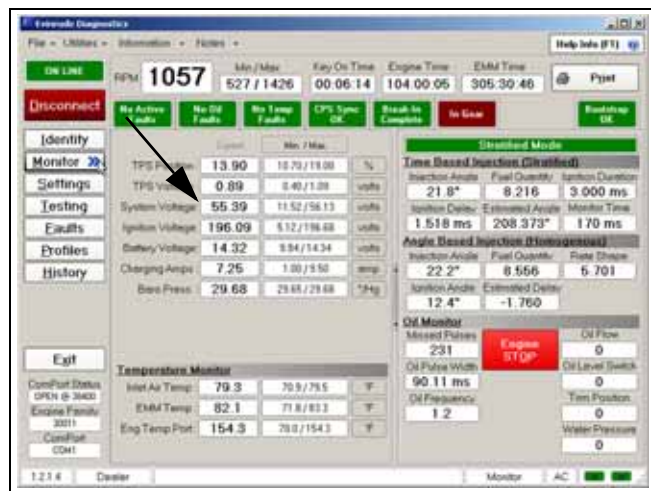
Engine Monitor Screen, System Voltage
